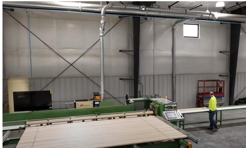
Factory assembly line for wall panels.
